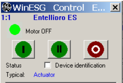
Figure 5-5: WinESG control panel contactor operation
