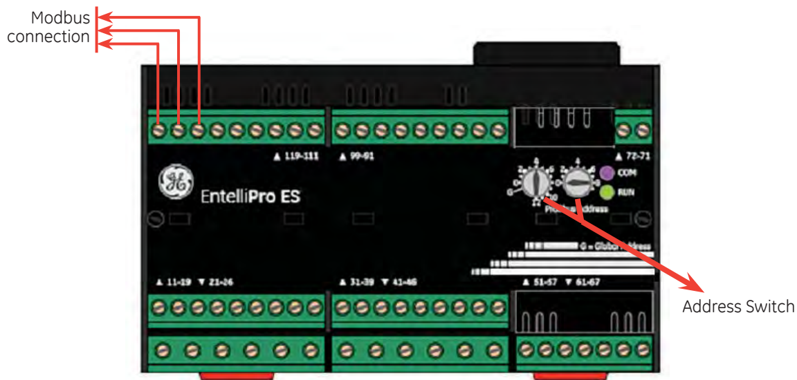
Figure 4-1: EntelliPro ES address switch settings and connection.
